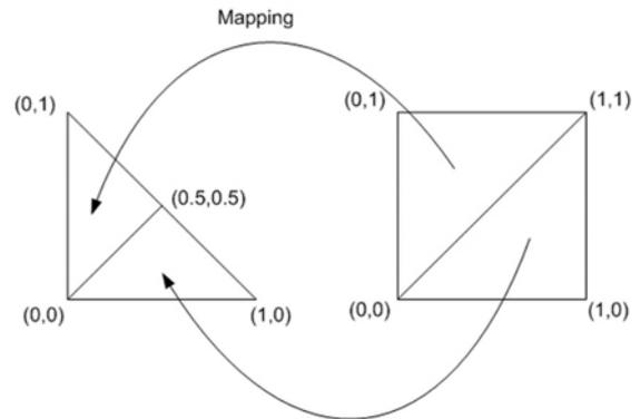
Figure 5. A schematic representation of the mapping between a square domain and a triangular domain.
